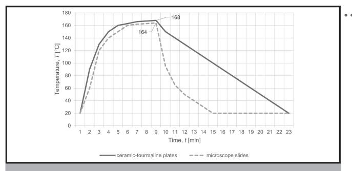
FIG. 8. Heating characteristics of the sample preparation system for UV-VIS spectrophotometric studies.
