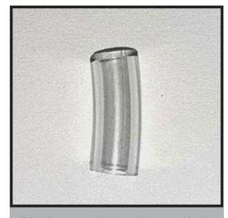
FIG. 5. Transparent drain sample prepared for the FTIR-ATR spectrophotometric study.
