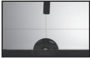
FIG. 9. Wettability study of drains by sessile drop method.
