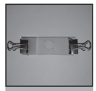
FIG. 7. Transparent drain sample prepared for UV-VIS absorption spectroscopy study.
